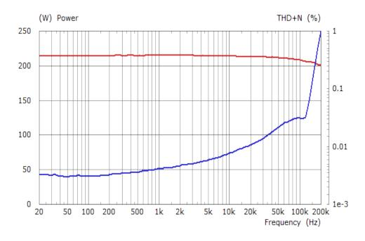
Input level normalized to max. output level at 200 kHz; THD+N < 1%
