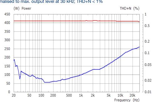
Input level normalised to max. output level at 30 kHz; THD+N < 1%
